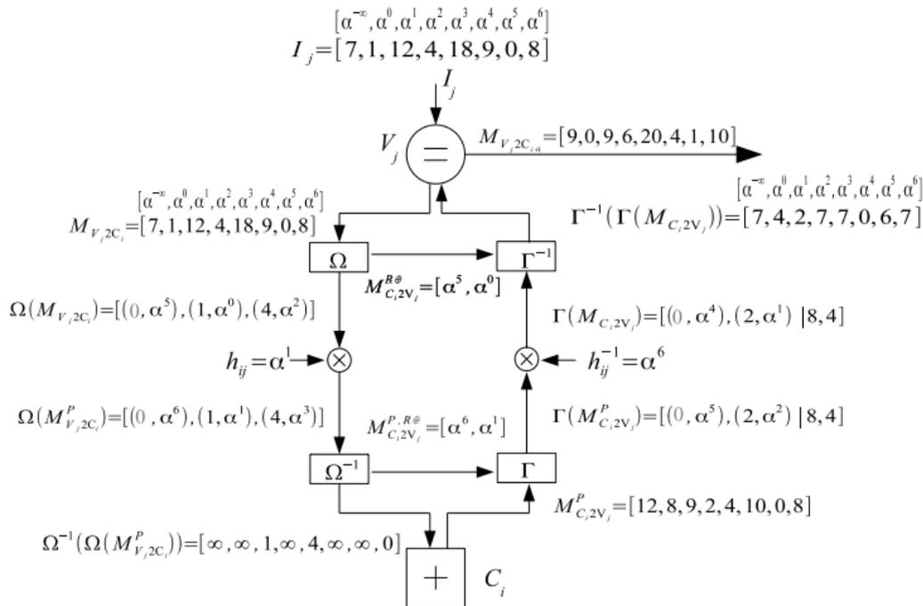
Figure 4: Toy Example of BRD Decoder on GF(8) with  $n_{vc} = 3$ ,  $n_B = 2$  and  $n_R = 2$
