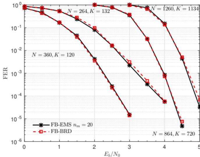
Figure 7: Simulation Results over GF(64) with AWGN and BPSK Modulation
