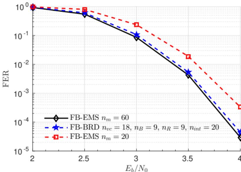
Figure 8: Simulation Results over GF(256) with AWGN and BPSK Modulation
