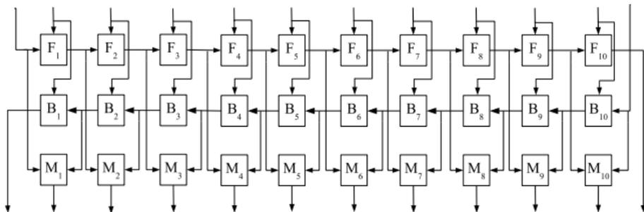
Figure 3: CN Decomposition in Forward-Backward Approach for  $d_c = 12$
