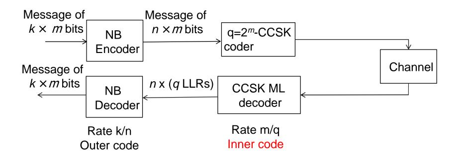
• The frame is composed of *N* segments of CCSK sequence (or symbol)
