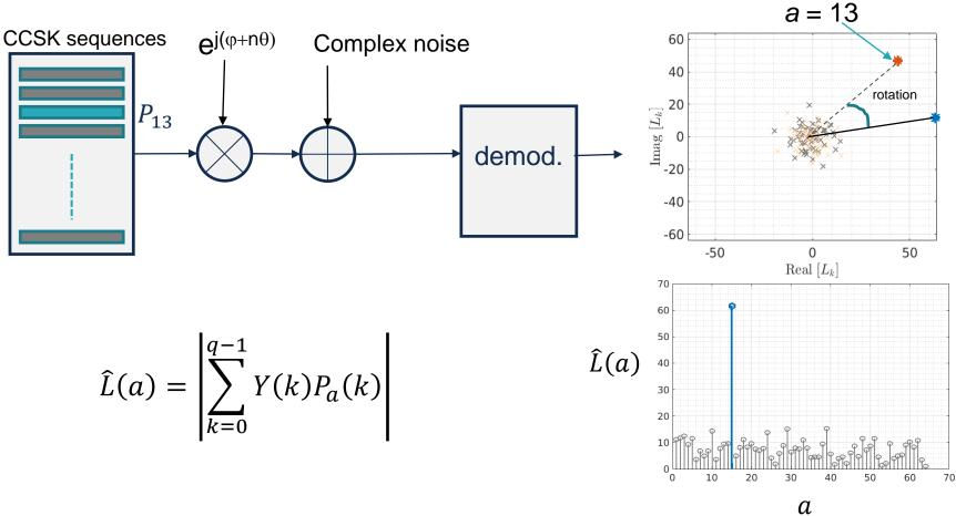
Phase and/or frequency offset require non-coherent demodulation.
