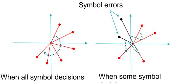
correct, the rotation pattern appears clearly and can be used for efficient detection. When some symbol decisions are wrong, the rotation pattern is completly « jammed »
