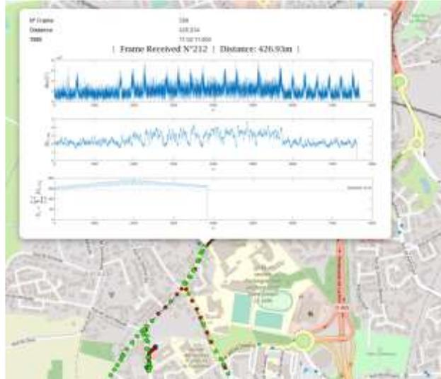
Figure 1: View of the interactive map showing a real-time QCSP frame transmission experiment in a mobile-radio urban environment (direct access to the map : [http://www-labsticc.univ-ubs.fr/~boutillon/QCSP\\_exp/index.html#15/47.7473/-3.3951](http://www-labsticc.univ-ubs.fr/~boutillon/QCSP_exp/index.html#15/47.7473/-3.3951)).
