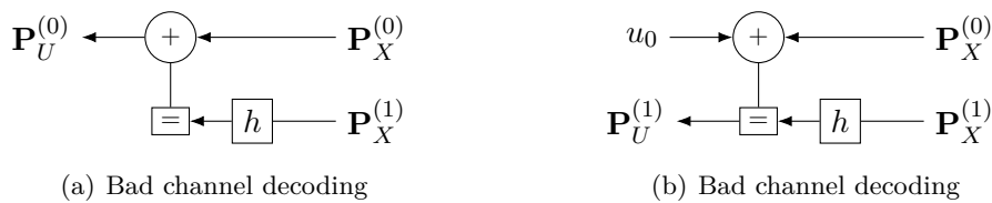
Figure 4.4: Decoding of bad and good virtual channels. For decoding the good channel, the decoder uses the knowledge of u_0 (genie-aided decoder), or an estimate of it, \hat{u}_0 (real-world decoder).
